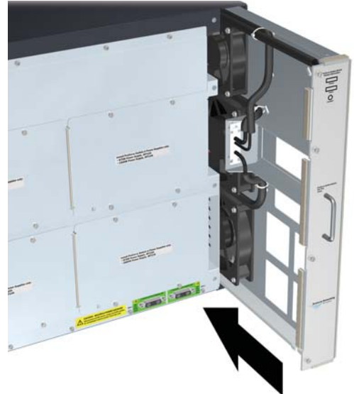
Figure 4. 8212zl Switch Fan Tray installation
