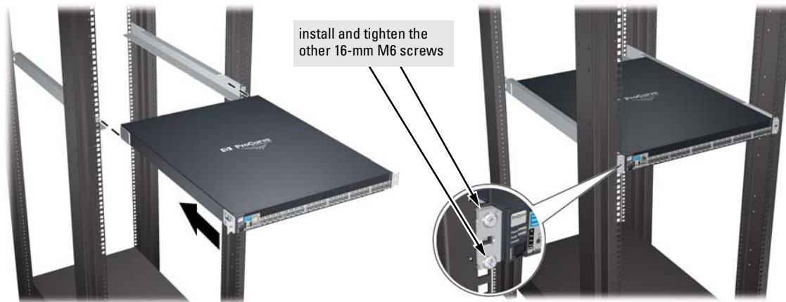
Figure 5. Sliding the Series 6600 switch into rails and installing mounting brackets screws
