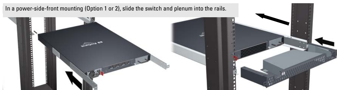
Figure 8. Installing a 6600 Switch in a Power-Side Mounting with an Air Plenum
