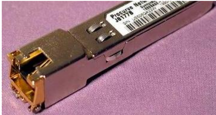
Figure 1. Latch in locked position
